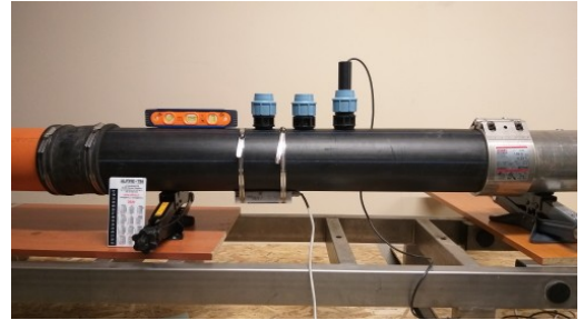
Test Rig „M-SIZE” for Open Channel flowmeters max. DN 160 / DN 200 / DN 250
