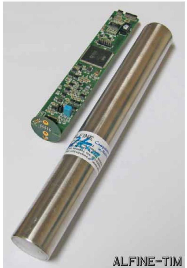
General view of flowmeter FLWM-10A and its electronics equipment
